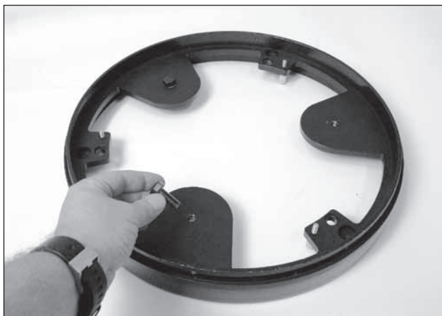
Figure 19. Thread the three counterweight mounting bolts into the holes in the rear end ring and tighten them firmly with a wrench.
