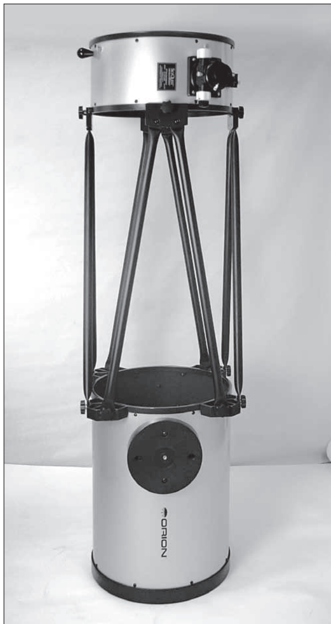
Figure 25. When the optical tube is assembled, the upper tube section should be oriented relative to the lower tube section as shown. Note the orientation of the focuser on the upper tube section relative to the side bearing on the lower tube section.
