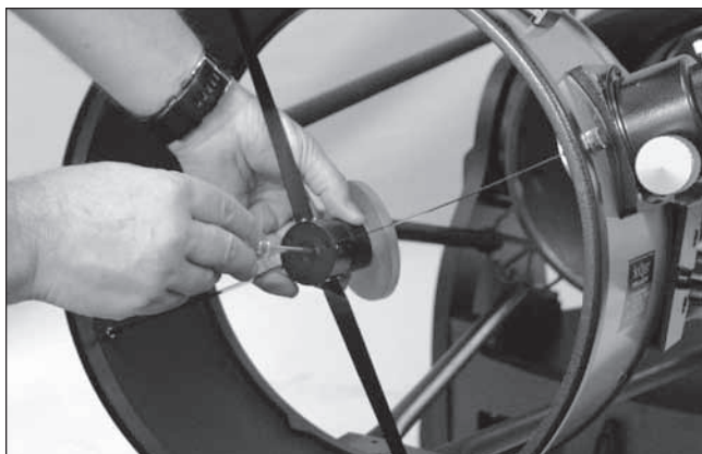
Figure 38. To center the secondary mirror axially under the focuser, hold the mirror holder in place with one hand while adjusting the center screw with a Phillips screwdriver.
