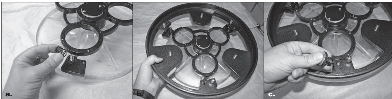
Figure 20. (a) Place the three springs on the exposed threaded shafts of the mirror cell. (b) Lower the rear end ring onto the mirror cell so that the threaded shafts of the mirror cell pass through the end ring, and the end ring rests on the springs. (c) Thread the collimation knobs, with nylon washers attached, through the rear end ring and onto the threaded shafts. Make sure the knobs have at least three full turns of engagement on the shafts.
