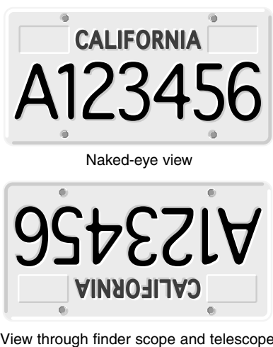
Figure 16. The view through a standard finder scope and reflector telescope is upside down. This is true for the SkyQuest IntelliScope and its finder scope as well.
