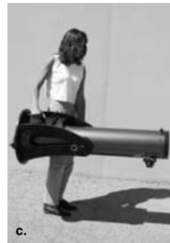
Figure 17. Picking up and carrying the SkyQuest IntelliScope as a single unit (with tube held captive on the base) requires some caution. (a) First, position the tube vertically. Then grasp the handle on the base with one hand while supporting the tube with the other. This ensures that the tube will not swing down and impact the ground (b) With knees bent, slowly lift the base while supporting the tube. (c) As you lift, continue to support the tube with one hand to keep it parallel with the ground. Make sure you are comfortable with the weight of the whole assembly before attempting the carry it!
