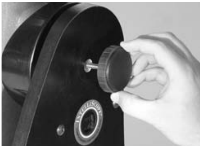
Figure 10. The tensioning knob, with the metal and nylon washers, goes on the side of the base with the IntelliScope port. The tensioning knob should be tightened until the CorrecTension pads just touch the telescope’s altitude bearing.
