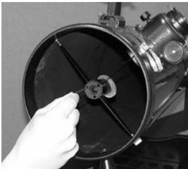
Figure 21. Adjust the tilt of the secondary mirror by loosening or tightening the three alignment set screws with a 2mm hex key.
