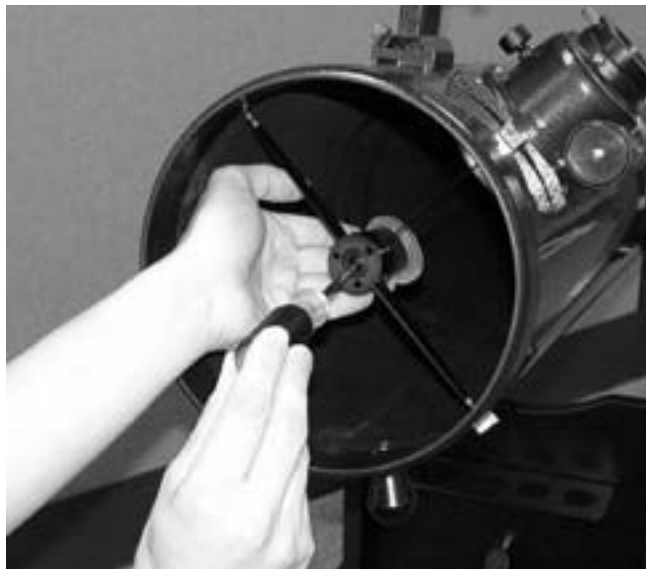
Figure 20. To center the secondary mirror under the focuser, hold the mirror holder in place with one hand while adjusting the center bolt with a Phillips screwdriver. Do not touch the mirror's surface!
