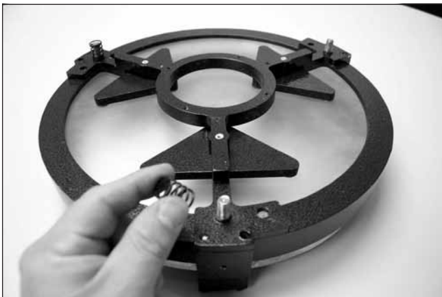
Figure 1.3. Place the three springs on the exposed threaded shafts of the mirror cell.
