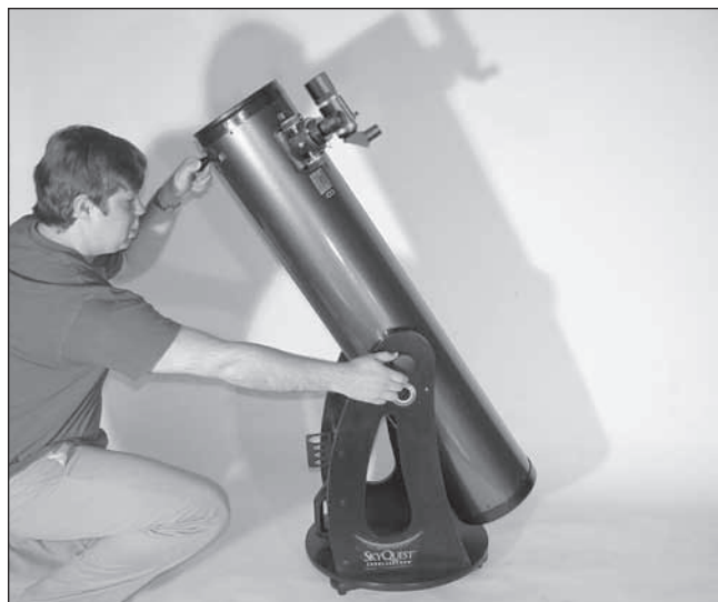
Figure 15. Adjust the tensioning knob until the altitude balance is just right. The telescope should move easily in altitude without drifting when you let go.
