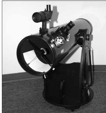
Figure 20. The SkyQuest XTi IntelliScope properly set up for collimation. Note the white paper placed across from the focuser, and the level angle of the optical tube. Ideally, the telescope should be pointing at a white wall.
