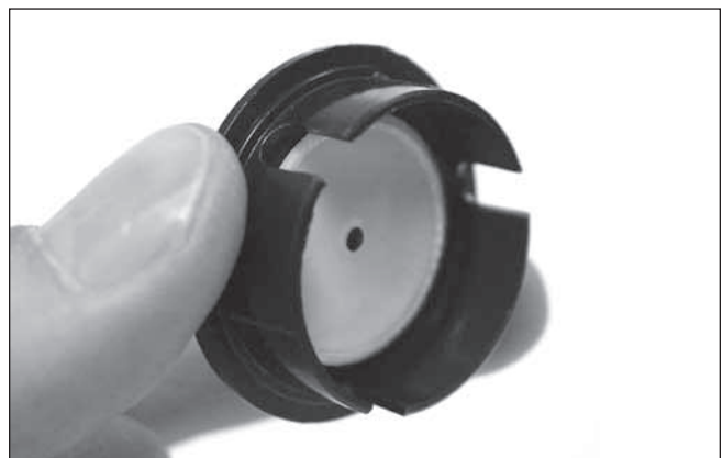
Figure 18. The quick collimation cap, which features a reflective inner surface, helps in centering reflections of the optics in the focuser during the collimation process.
