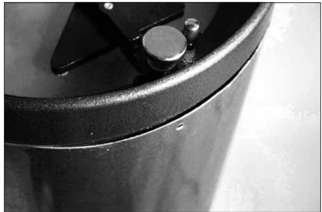
Figure 1.7. Locate the area of tube that is bulging out and preventing the mirror cell from fully seating.
