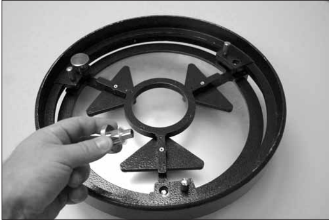
Figure 1.5. Thread the collimation thumbnuts, with nylon washers attached, through the rear end ring and onto the threaded shafts. Make sure the thumbnuts have at least three full turns of engagement on the shafts.
