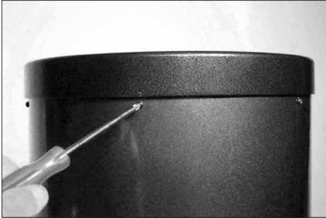
Figure 1.2. To remove the rear end ring, unthread the screws that connect it to the tube.
