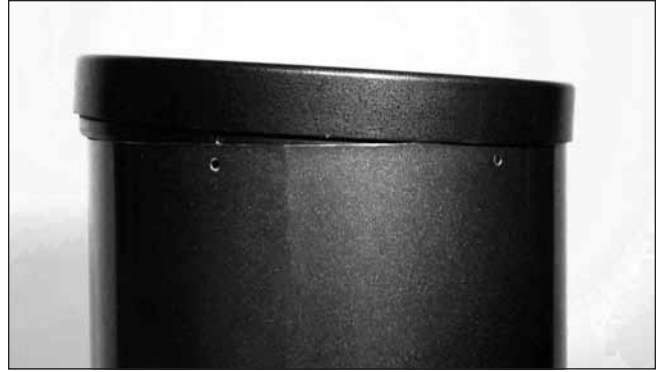
Figure 1.6. Lower the assembled mirror cell onto the tube so one side of the end ring is seated on the tube edge. The threaded attachment holes in the end ring should also be lined up with the through holes in the end of the tube.
