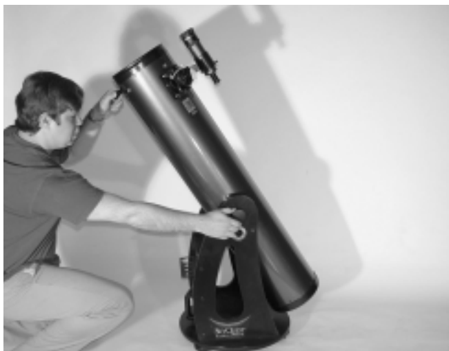
Figure 15. Adjust the tensioning knob until the altitude balance is just right. The telescope should move easily in altitude without drifting when you let go.
