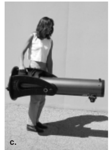
Figure 17. Picking up and carrying the SkyQuest IntelliScope as a single unit (with tube held captive on the base) requires some caution. (a) First, position the tube vertically. Then grasp the handle on the base with one hand while supporting the tube with the other. This ensures that the tube will not swing down and impact the ground (b) With knees bent, slowly lift the base while supporting the tube. (c) As you lift, continue to support the tube with one hand to keep it parallel with the ground. Make sure you are comfortable with the weight of the whole assembly before attempting the carry it!
