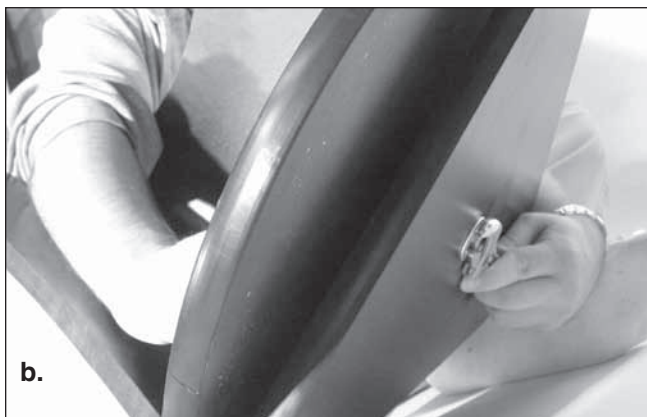
Figure 4. To connect the baseplates, tilt them only slightly, as shown. Do not place them on their side. (a) Use one wrench to hold the hex nut steady (b) while turning the other end of the azimuth axis screw.
