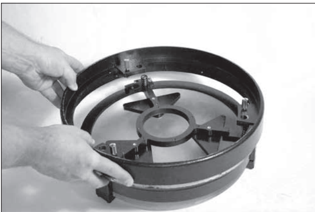
Figure 1.4. Lower the rear end ring onto the mirror cell so that the threaded shafts pass through the end ring, and the end ring rests on the springs.
