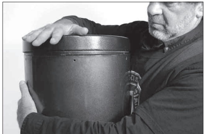
Figure 1.8. Hug the tube so that your chest pushes against the bulge, and a gentle tap should fully seat the mirror cell onto the tube.
