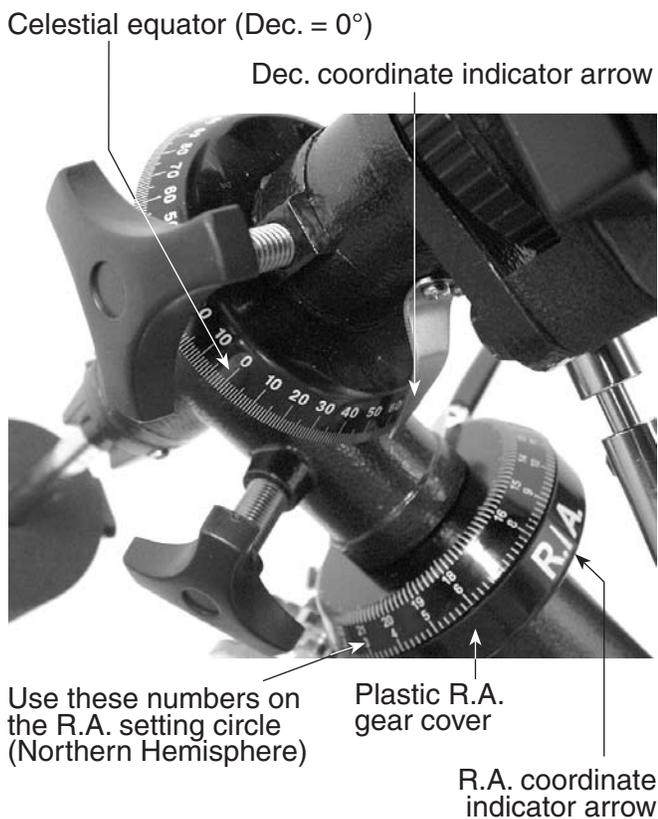
**Figure 5: For Northern Hemisphere observers, use the lower set of numbers on the R.A. setting circle. The R.A. coordinate indicator arrow is between the “R” and the “A” on the plastic gear cover. The telescope (not shown) is pointing north of the celestial equator, so the approximate coordinates of the mount in the image are R.A. 8h 30m Dec. 60°.**
