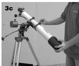
Figure 3A, 3B, 3C, 3D: Proper operation of the equatorial mount requires balancing the telescope tube on the R.A. axis. (a) With the R.A. lock knob released, slide the counterweight along the counterweight shaft until it just counterbalances the tube. (b) When you let go with both hands, the tube should not drift up or down. (c) With the Dec. lock knob released, loosen the tube ring lock clamps a few turns and slide the telescope forward or back in the tube rings. (d) When the tube is balanced about the Dec. axis, it will not move when you let go.
