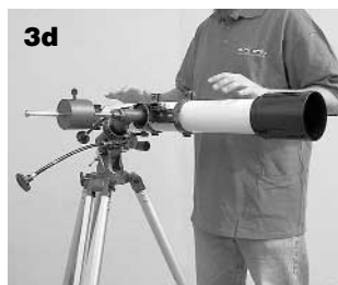
Figure 3A, 3B, 3C, 3D: Proper operation of the equatorial mount requires balancing the telescope tube on the R.A. axis. (a) With the R.A. lock knob released, slide the counterweight along the counterweight shaft until it just counterbalances the tube. (b) When you let go with both hands, the tube should not drift up or down. (c) With the Dec. lock knob released, loosen the tube ring lock clamps a few turns and slide the telescope forward or back in the tube rings. (d) When the tube is balanced about the Dec. axis, it will not move when you let go.
