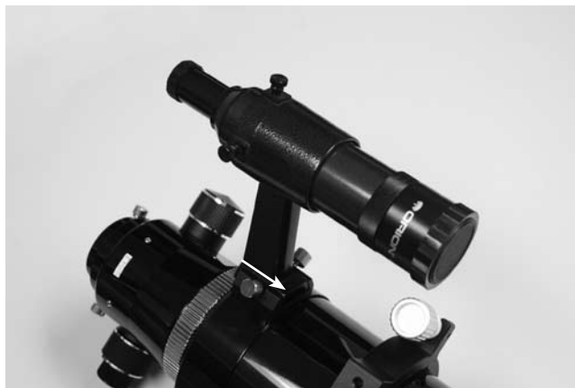
Figure 6. Slide the finder scope bracket into the finder scope dovetail base and secure the locking thumbscrew(s).
