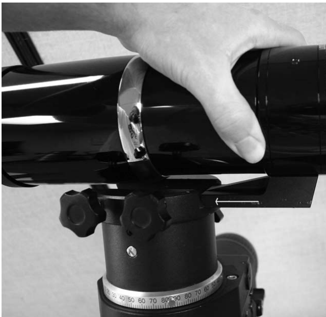
Figure 8. Align the mounting block with the dovetail holder and slide it forward. Tighten the attachment screw(s) on the dovetail holder of the mount.
