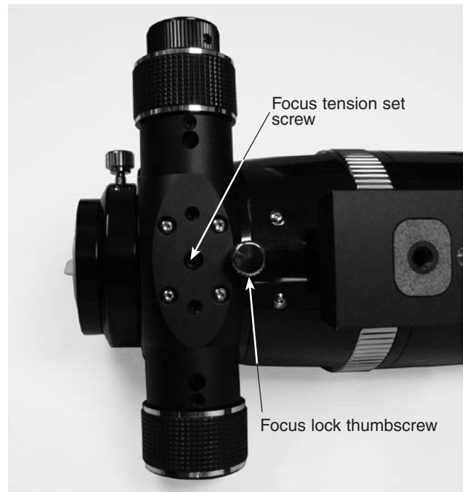
Figure 3. Adjustments can be made to the focus tension set screw using the provided 2.5mm hex key. Tightening the focus lock thumbscrew will stop the focuser drawtube from moving.
