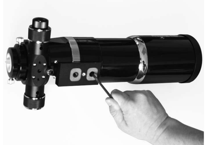
Figure 9. For a greater range of balance on the EON 72mm and 80mm, switch the direction of mounting block using a 4mm hex key.
