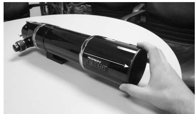
Figure 2. Gently pull the dew shield outward until it stops.
