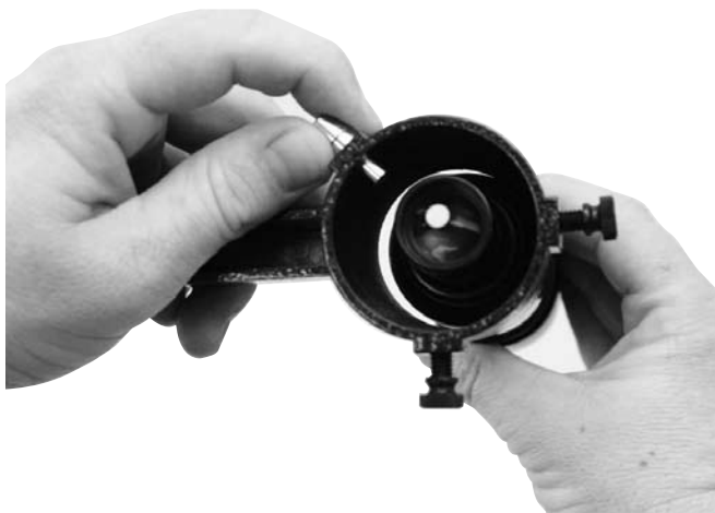
Figure 3b. Pull-back on the tensioner and slide the finder scope into its bracket until the O-ring is seated in the bracket ring.
