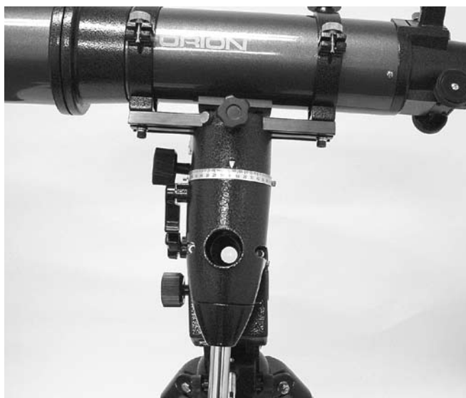
Figure 12. The optical tube must be at a 90° angle to the right ascension axis in order to view through the polar axis finder.
