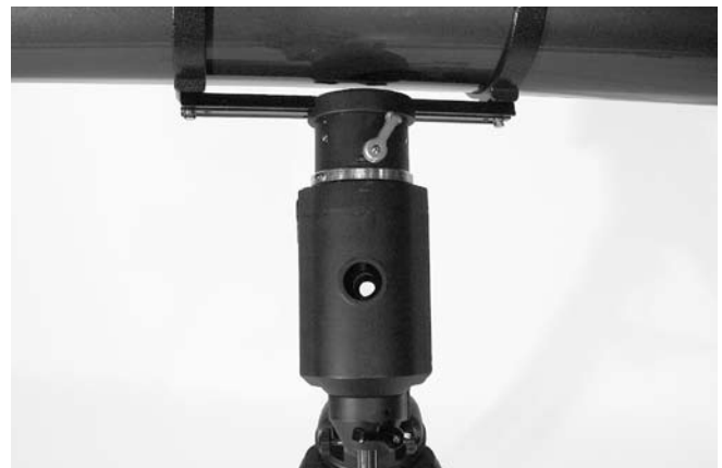
Figure 8. The optical tube must be rotated about the declination axis in order to view through the polar axis finder.
