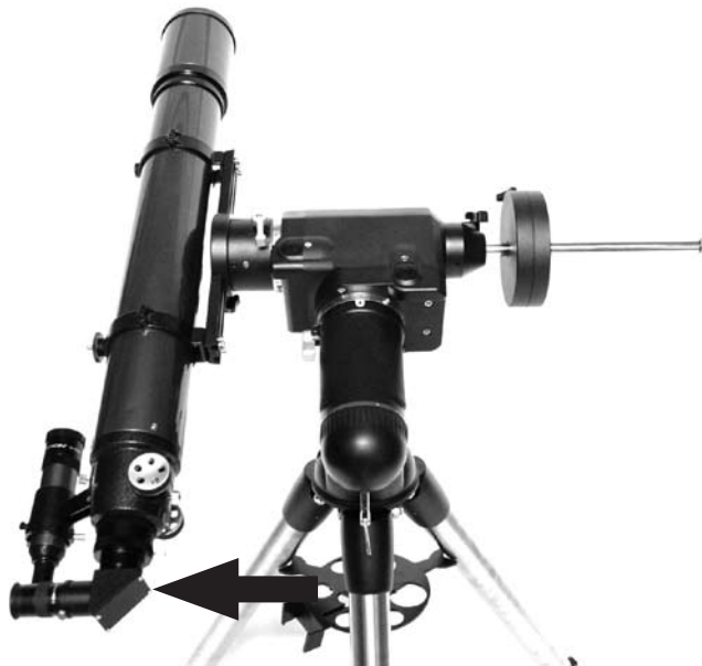
Figure 19. gently push the telescope horizontally to determine direction of optical axis offset.
