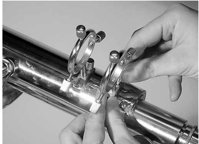
Figure 4. Attaching the finder scope brackets to the optical tube.
