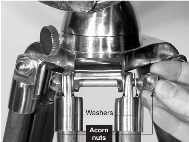
Figure 2. Attaching the tripod legs to the mount.
