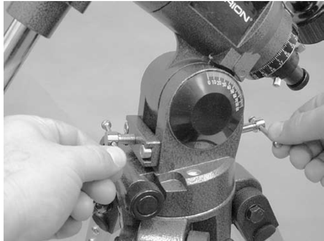
Figure 2: To adjust the latitude angle of the equatorial mount, loosen one of the two latitude adjustment T-bolts, then tighten the other.
