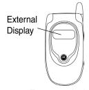
When your phone is turned on and the flip is closed, the external display shows the phone status, including battery and network signal status. It also shows the time. When you receive an incoming call, the external display shows the caller's number or
