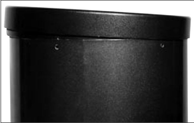
Figure 6. Lower the assembled mirror cell onto the tube so one side of the end ring is seated on the tube edge. The threaded attachment holes in the end ring should also be lined up with the through holes in the end of the tube
