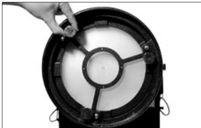
Figure 23. The tilt of the primary mirror is adjusted by turning one or more of the three spring-loaded collimation thumb screws.
