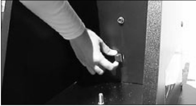
Figure 10. Position the rubber bumper “stop” over the index mark on the inside surface of the front brace.
