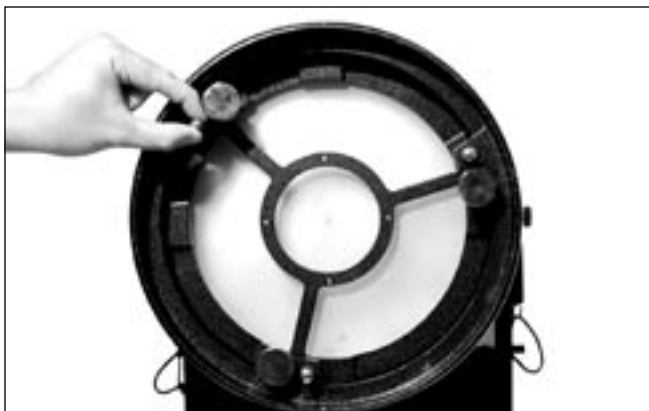
Figure 22. The three thumb screws that lock the primary mirror in place must first be loosened before any adjustments can be made.
