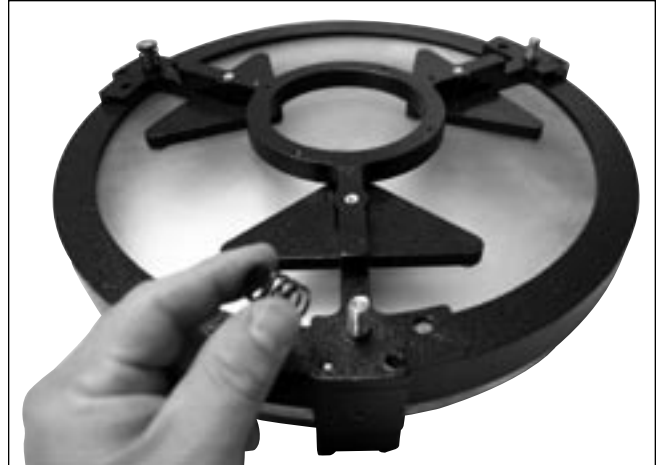
Figure 3. Place the three springs on the exposed threaded shafts of the mirror cell.
