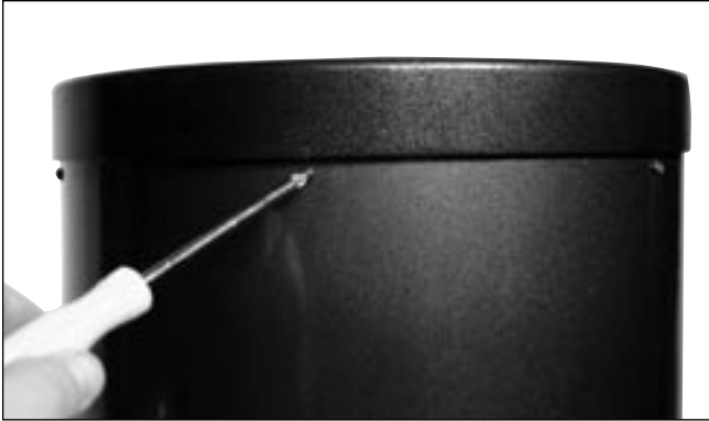
Figure 2. To remove the rear end ring, unthread the six screws that connect it to the tube.
