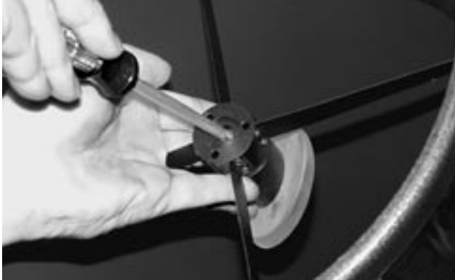
Figure 20. To center the secondary mirror under the focuser, hold the secondary mirror holder in place with your fingers while adjusting the center screw with a Phillips screwdriver. Do not touch the mirror's surface!
