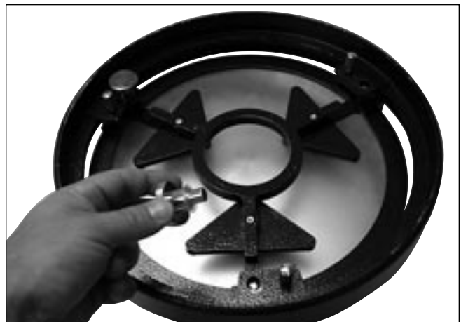
Figure 5. Thread the collimation thumbnuts, with nylon washers attached, through the rear end ring and onto the threaded shafts. Make sure the thumbnuts have at least three full turns of engagement on the shafts.
