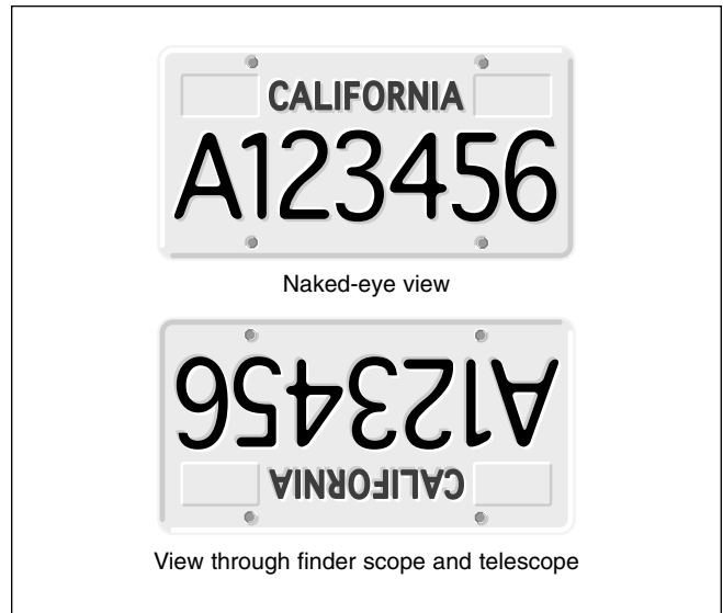
Figure 18. The view through a standard finder scope and a reflector telescope is upside down. This is true for the SkyQuest and its finder scope as well.
