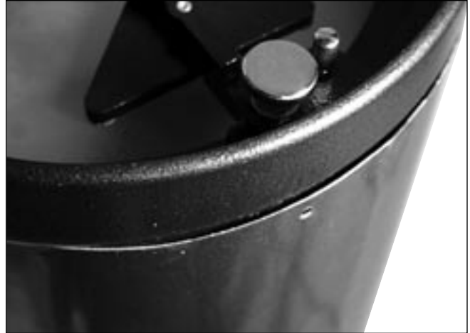
Figure 7. Locate the area of tube that is bulging out and preventing the mirror cell from fully seating.
