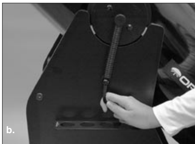
Figure 14. (a) To attach the spring to the base, grip the pull loop with your index finger and pull down on the spring. (b) While pulling down, slip the end ring of the spring over the screw head and onto the narrow part of the nylon spacer, then release the pull loop.
