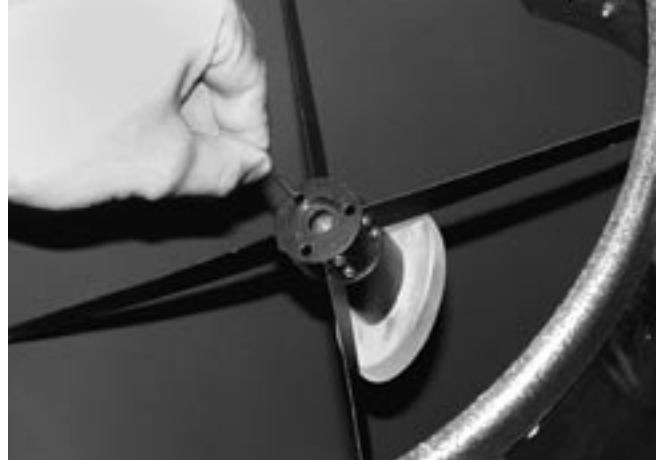
Figure 21. Adjust the tilt of the secondary mirror by loosening or tightening the three alignment screws with a 2mm hex key.
