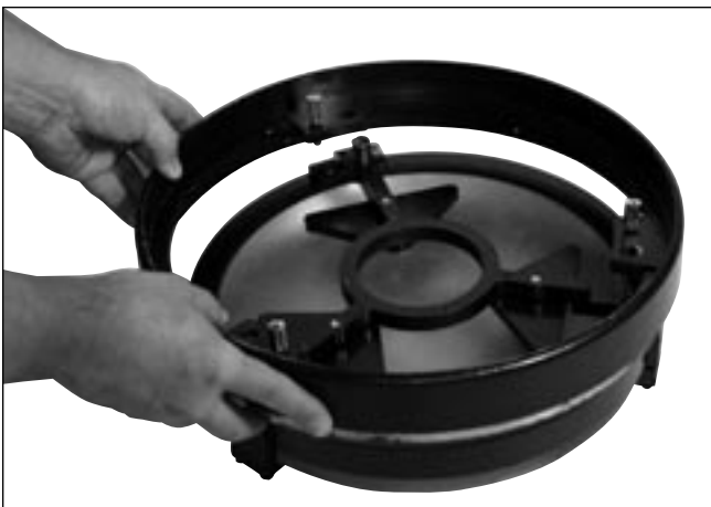
Figure 4. Lower the rear end ring onto the mirror cell so that the threaded shafts pass through the end ring, and the end ring rests on the springs.
