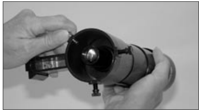
Figure 15b. Pull back on the tensioner and slide the finder scope into its bracket until the O-ring is seated in the bracket ring.
