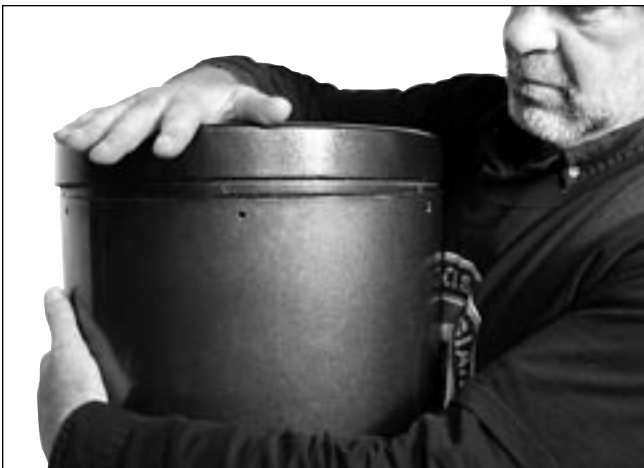
Figure 8. Hug the tube so that your chest pushes against the bulge, and a gentle tap should fully seat the mirror cell onto the tube.
