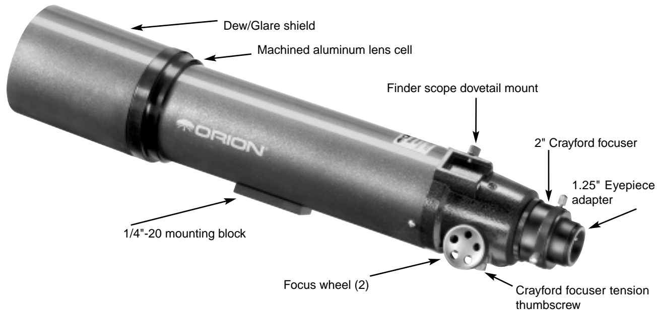
Figure. The 80mm f/7.5 ED Refractor optical tube assembly
