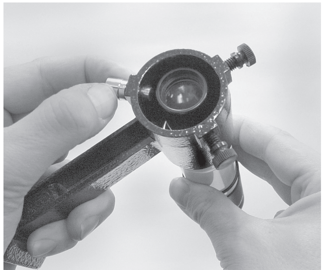
Figure 2b. Inserting the finder scope into the finder scope bracket.
