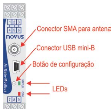
Figura 4 - Painel frontal AirGate-Modbus .
