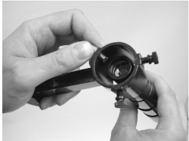
Figure 2b. Pull back on the tensioner and slide the finder scope into its bracket until the O-ring is seated in the bracket ring
