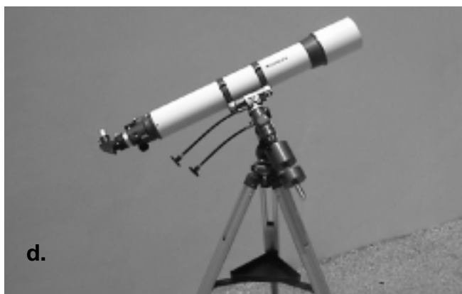
Figure 10. This illustration shows the telescope pointed in the four cardinal directions: (a) north, (b) south, (c) east, (d) west. Note that the tripod and mount have not been moved; only the telescope tube has been moved on the R.A. and Dec. axes.
