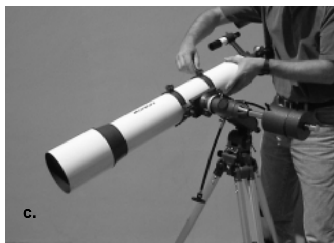
Figure 5. Proper operation of the equatorial mount requires that the telescope tube be balanced on both the R.A. and Dec. axes. (a) With the R.A. lock lever released, slide the counterweights along the counterweight shaft until they just counterbalance the tube. (b) When you let go with both hands, the tube should not drift up or down. (c) With the Dec. lock lever released, loosen the tube ring lock clamps a few turns and slide the telescope forward or back in the tube rings. (d) When the tube is balanced about the Dec. axis, it will not move when you let go.
