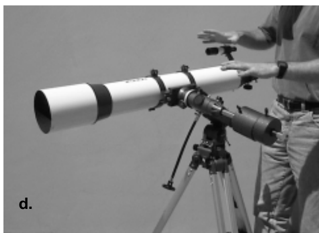
Figure 5. Proper operation of the equatorial mount requires that the telescope tube be balanced on both the R.A. and Dec. axes. (a) With the R.A. lock lever released, slide the counterweights along the counterweight shaft until they just counterbalance the tube. (b) When you let go with both hands, the tube should not drift up or down. (c) With the Dec. lock lever released, loosen the tube ring lock clamps a few turns and slide the telescope forward or back in the tube rings. (d) When the tube is balanced about the Dec. axis, it will not move when you let go.
