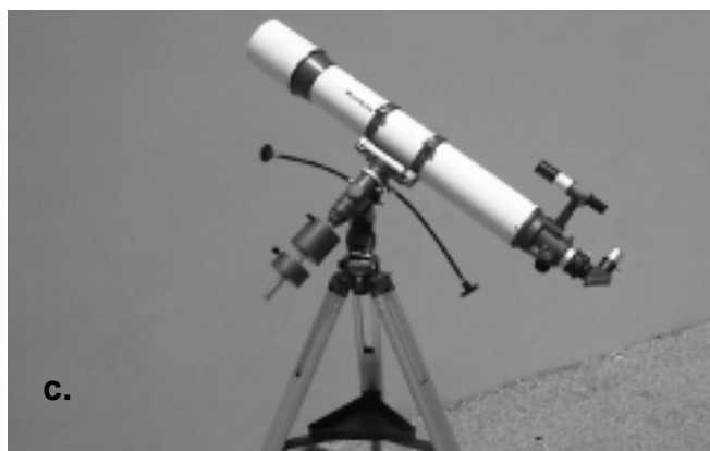
Figure 10. This illustration shows the telescope pointed in the four cardinal directions: (a) north, (b) south, (c) east, (d) west. Note that the tripod and mount have not been moved; only the telescope tube has been moved on the R.A. and Dec. axes.
