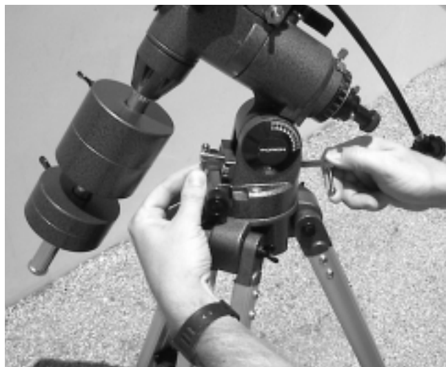
Figure 2. To adjust the latitude angle of the equatorial mount, loosen one of the two latitude adjustment T-bolts, then tighten the other.
