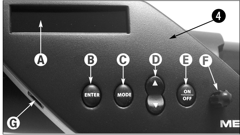
Fig. 3: Detailed view of the NGC computer control panel.
