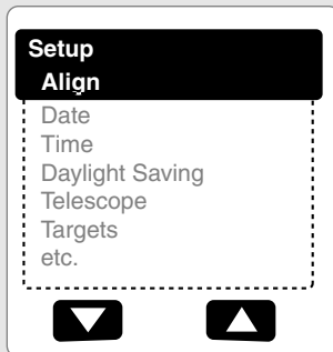
Fig. 20: Menu options display on the second line. Use the Scroll keys to move up or down through the list of options. Press ENTER to select the desired option.
