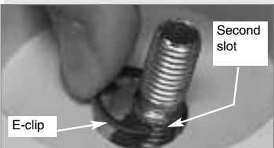
Fig. 5b: Snap e-clip all the way onto shaft above mount (shown partially attached).
