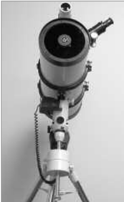
Fig. 16a: The polar home position, front view.
