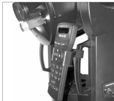
Fig. B: Handbox holder attached to fork arm handle. Adjust holder to a convenient tilt.
