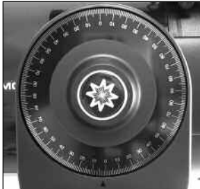
Fig. 31: Section of Declination Setting Circle.
