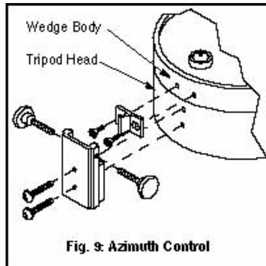
3. Attach the Azimuth Base to the Field Tripod using the 2 ea. 8-32 x 1" round-head machine screws.
