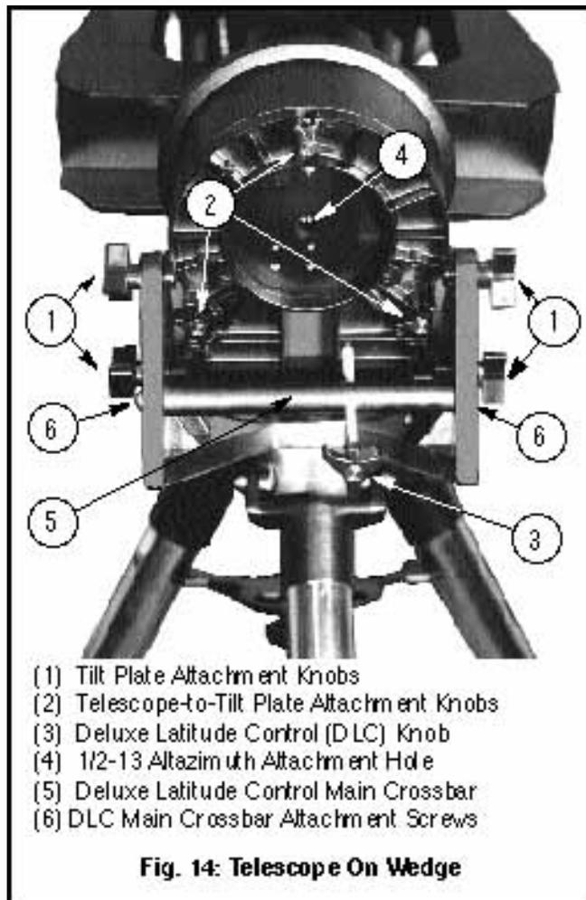
**Fig. 14: Telescope On Wedge**
