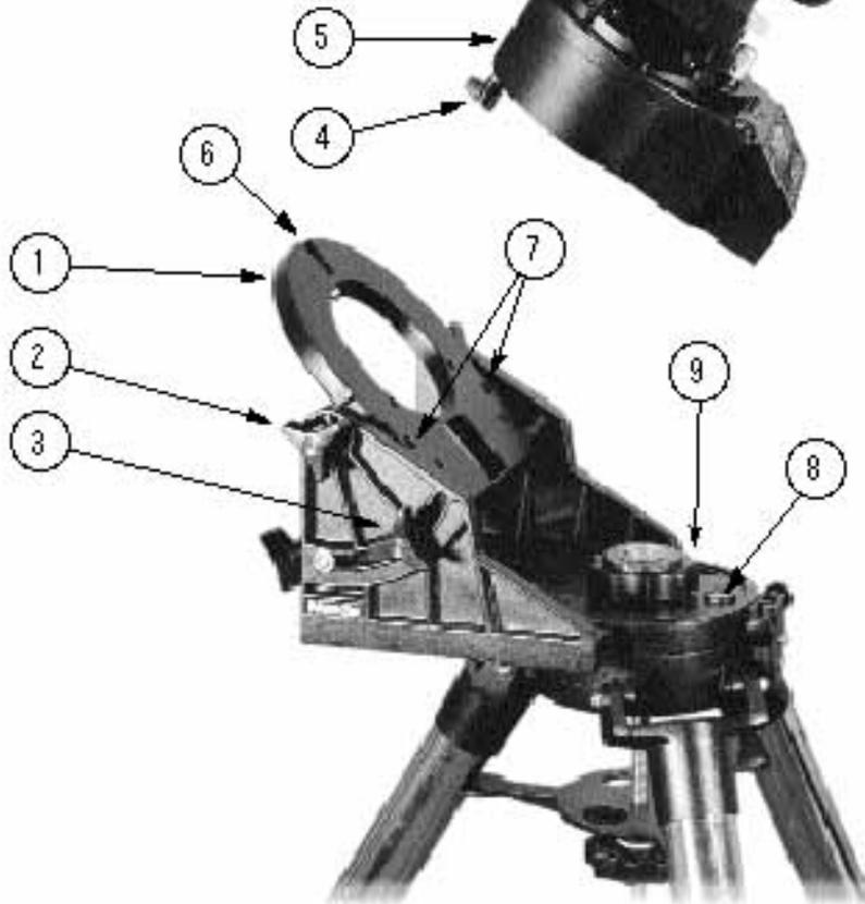
**Fig. 12: Placing the Telescope on the Equatorial Wedge**
