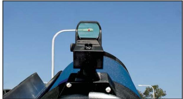
The Red Dot Finder has been aligned at the factory, but you may need to touch-up the alignment from time to time. To do this, look through the eyepiece of your scope and using the hand controller center a distant object. Now turn on the Red Dot Viewfinder and adjust the brightness so you can see the red dot. Look through the sight as pictured above.
