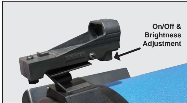
Because your telescope has so much magnification, its field of view is very small. This can make it hard to know exactly where your telescope is pointing by simply looking at it. To help you point the telescope quickly and accurately, for terrestrial targets or GO TO pointing, the LT Series has a 1X Red Dot Viewfinder.
