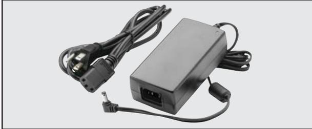
**Universal AC Adapter (07584):** This adapter supplies a constant regulated 12 volt DC at up to 5 Amps from either a standard 115 volt AC or 220 volt AC household supply. It is the only tested and recommended AC power supply for the LT Series system.
