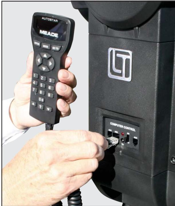
**8** Be sure the telescope master power switch is in the off position. Remove the LT Series handbook and the coiled interface cable from the packing materials. Plug one end into the HBX port of the control panel and plug the other end into the Handbox port on the LT Series handbook.
