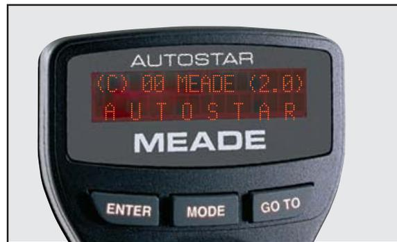
**11** Flip the Power Switch on the computer control panel to the ON position. The copyright message lights on AutoStar's LCD display.
