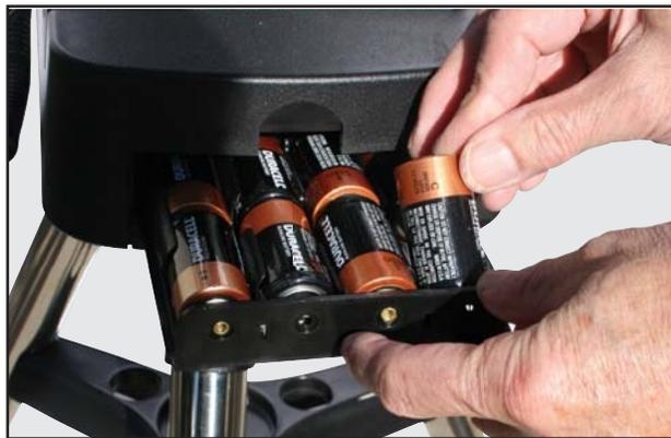
**6** Remove the end cover from the battery compartment exposing the battery tray. Carefully slide the battery tray out until it reaches its end stop. Insert 8 (user supplied) Alkaline "C" batteries into the battery compartment. Take care that the batteries + and - ends are as indicated in the battery holder.
