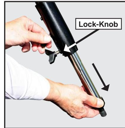
**3** Thread in two lock-knobs on each leg (six total) near the foot of each tripod leg. Use the lock-knobs to vary the height of the inner, extendible tripod leg sections. Tighten the locks to a firm feel only; do not overtighten.
