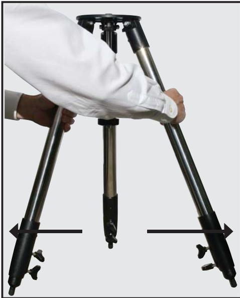
**2** Remove the field tripod from the shipping carton. Stand the tripod vertically with the tripod feet down and with the tripod still fully collapsed. Grasp two of the tripod legs and, with the full weight of the tripod on the third leg, gently pull the legs apart to a fully open position.
