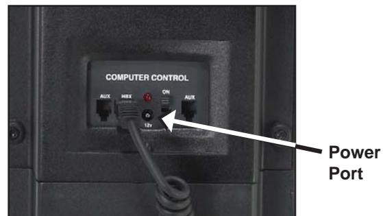
**7** Use only the optional Meade Universal AC Power Adapter (part number 07584 for North America or 07584F for 220v foreign) with your LT Series telescope when connecting to AC power. It is specifically selected to provide the quality voltage and current required to power and protect the electronics in the telescope. Power adapters from other manufactures may cause damage and void your warranty.
