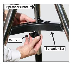
Remove the end nut from the spreader shaft and slide the spreader in between the telescope legs. Attach the end nut and hand tighten until the telescope legs are held snuggly in the most spread position. Position the tripod where you want the telescope to be and check that the top of the tripod is approximately level.
