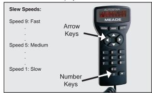
"Press 0 to align or Mode for Menu" displays. You can use the Arrow keys to slew (move) the telescope up, down, right, or left. To change the telescope's slew speed, press a Number key. "9" is the fastest speed and "1" is the slowest speed. See page 20 for more details. Or you can Press "0" to begin Easy Alignment. See page 11 for more information.
