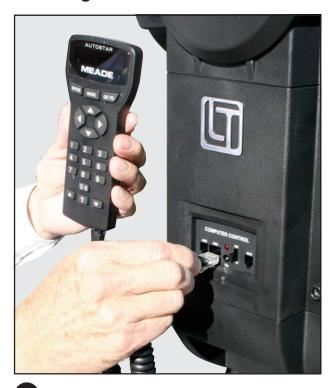
Be sure the telescope master power switch is in the off position. Remove the LT Series handbox and the coiled interface cable from the packing materials. Plug one end into the HBX port of the control panel and plug the other end into the Handbox port on the LT Series handbox.
