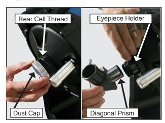
9 Remove the dust cap from the rear cell of the telescope. Thread the 1.25" eyepiece holder onto the rear cell thread. Slide the diagonal prism into the eyepiece holder and lock in place by turning the thumbscrew to a firm feel. Place the Super Plössl 26mm eyepiece into the diagonal prism and tighten the diagonal prism thumbscrew to a firm feel only.
