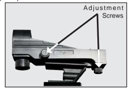
Now, without moving the telescope, adjust the indicated thumb screws until you have put the red dot on the object at which you were looking. It's that simple.
