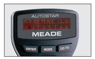
Flip the Power Switch on the computer control panel to the ON position. The copyright message lights on AutoStar's LCD display.
