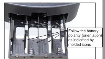
CAUTION: Use care to install batteries as indicated by the battery compartment. Follow battery manufacturer's precautions. Do not install batteries backwards or mix new and used batteries. Do not mix battery types. If these precautions are not followed, batteries may explode, catch fire, or leak. Improperly installed batteries void your Meade warranty. Always remove the batteries if they will not be used for a long period of time.
