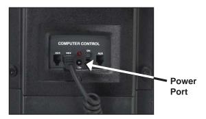
Use only the optional Meade Universal AC Power Adapter (part number 07584 for North America or 07584F for 220v foreign) with your LT Series telescope when connecting to AC power. It is specifically selected to provide the quality voltage and current required to power and protect the electronics in the telescope. Power adapters from other manufactures may cause damage and void your warranty.
