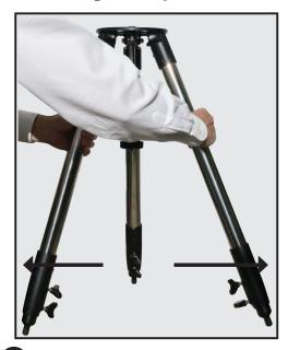
Remove the field tripod from the shipping carton. Stand the tripod vertically with the tripod feet down and with the tripod still fully collapsed. Grasp two of the tripod legs and, with the full weight of the tripod on the third leg, gently pull the legs apart to a fully open position.
