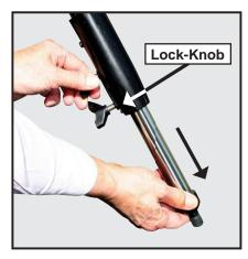
Thread in two lock-knobs on each leg (six total) near the foot of each tripod leg. Use the lock-knobs to vary the height of the inner, extendible tripod leg sections. Tighten the locks to a firm feel only; do not overtighten.
