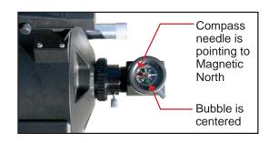
Figure 7: Bubble Level/Compass
