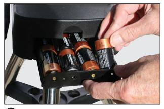
6 Remove the end cover from the battery compartment exposing the battery tray. Carefully slide the battery tray out until it reaches its end stop. Insert 8 (user supplied) Alkaline "C" batteries into the battery compartment. Take care that the batteries + and - ends are as indicated in the battery holder.
