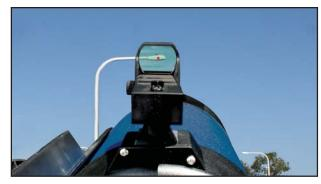
The Red Dot Finder has been aligned at the factory, but you may need to touch-up the alignment from time to time. To do this, look through the eyepiece of your scope and using the hand controller center a distant object. Now turn on the Red Dot Viewfinder and adjust the brightness so you can see the red dot. Look through the sight as pictured above.
