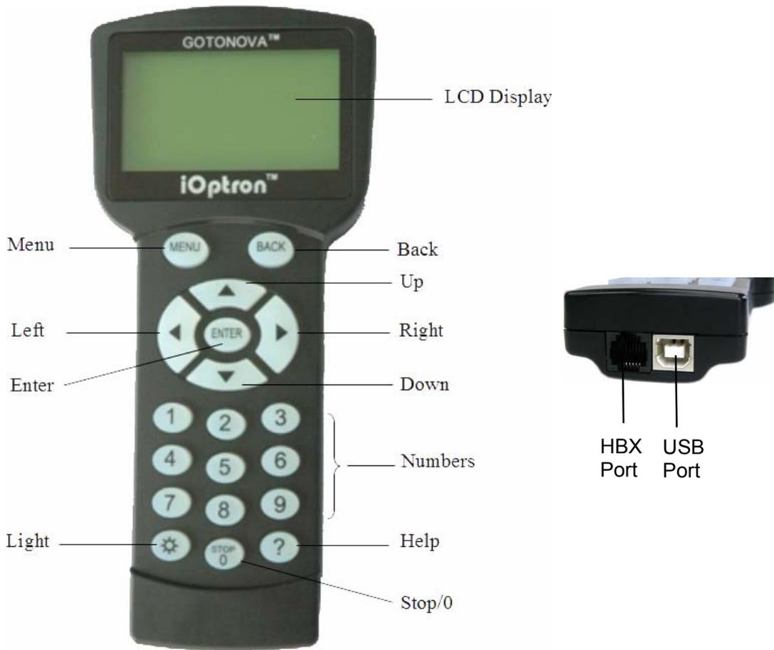
Figure 1. GoToNova 8401 Hand Controller
