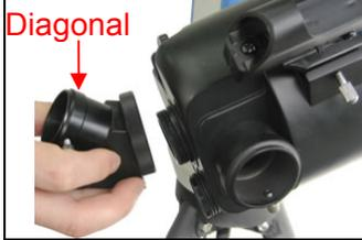
Install **Diagonal** by screwing it onto the back end of the scope. You can adjust the position of the diagonal by loosening the free-spinning threader on the diagonal.
