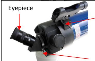
Install the **Finderscope** by sliding the dovetail plate onto the sleeve (see arrow) and tightening the side screw.
