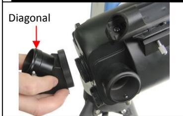
Install **Diagonal** by screwing it onto the back end of the scope. You can adjust the position of the diagonal by loosening the free-spinning threader on the diagonal.
