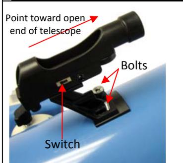
**Attach the red dot finder scope to the telescope tube (#1):**
