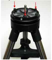
5. Remove iEQ center stud and alignment peg. Insert the MiniTower Securing Bolt through the hole on the top mounting flange. Install the Turning Lever.
