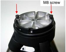
3. Put the MiniPier body onto the Base Flange and secure it using three locking screws.
