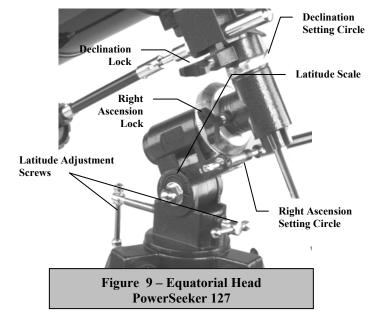
Remember, while Polar aligning, do NOT move the telescope in R.A. or DEC. You do not want to move the telescope itself, but the polar axis. The telescope is used simply to see where the polar axis is pointing.
