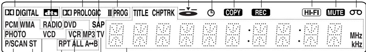
Indicates clock, total playing time, elapsed time, remaining time, title number, chapter/track number, channel, radio frequency, level, volume, channel or current deck status (Playback, Pause, Mode, etc).
