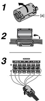
Be sure to attach the ferrite core to the speaker cables (for connecting to this unit).
