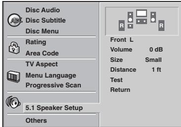
1. Select "5.1 Speaker Setup" using the ▲/▼ buttons on the setup menu.
