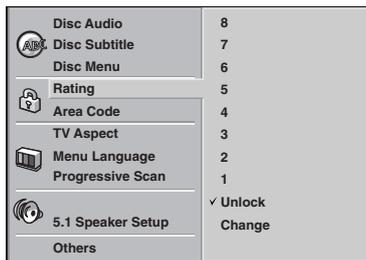
1. Select **Rating** on the Setup menu using **▲/▼** buttons in stop mode.
