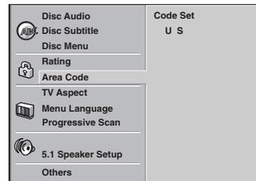
1. Select **Area Code** using the **▲/▼** buttons on the setup menu.
