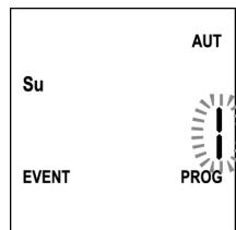
5. Select the event (1 to 5) using the **UP / DOWN** keys and press the  **MENU** key to confirm.
