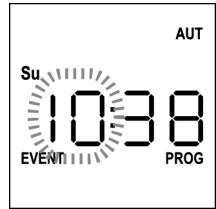
6. Set the time using the **UP** and **DOWN** keys and press the  **MENU** key to confirm. The minute digits blink:
