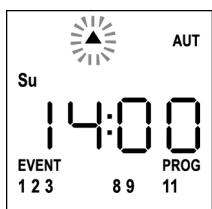
11. Select the desired event using the **UP** and **DOWN** keys and press **MENU** to confirm and proceed.
