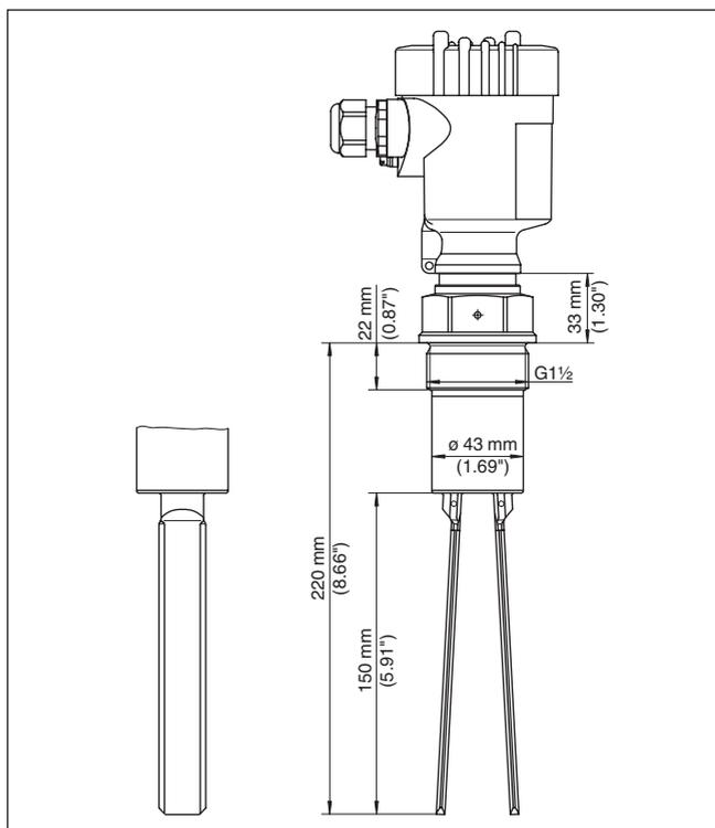
Fig. 52: VEGAWAVE 61 - Modelo com rosca G1½ A (DIN ISO 228/1)
