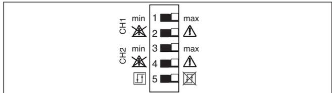
Fig. 3: Interruptor DIL VEGATOR 112
