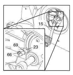
Slide the Reed Switch slightly closer to or away from the Magnet. Then, retighten the Screw. Turn the Crank Arm for a moment. Repeat until the console displays correct feedback. When the Reed Switch is correctly adjusted, reattach the Pedal Guard (8) and the left Side Shield Cover (14).
