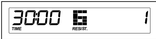
After a few seconds, a profile of the resistance levels of the workout will scroll across the center display.
