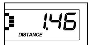
Note: The console can show pedaling speed and distance in either miles or kilometers. To change the unit of measurement, see THE USER MODE on page 17.
