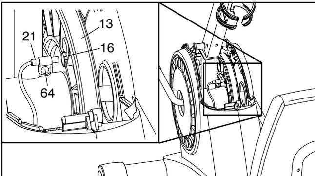
Slide the Reed Switch (21) slightly closer to or away from the Pulley Magnet (16), and then retighten the M4 x 15mm Screw (64). Turn the Pulley (13) for a moment. Repeat these actions until the console displays correct feedback.
