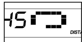
**The right display**—This display can show the distance you have pedaled in miles or kilometers and your pedaling pace in miles per hour or kilometers per hour. The display will change modes every few seconds.
