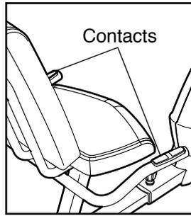
When your pulse is detected, a heart-shaped symbol will flash in the display and then your heart rate will be shown. For the most accurate heart rate reading, hold the contacts for at least 15 seconds.
