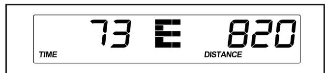
The center display will show the selected unit of measurement. An E for English miles or an M for metric kilometers will appear in the display. To change the unit of measurement, press the Resistance increase button repeatedly.
