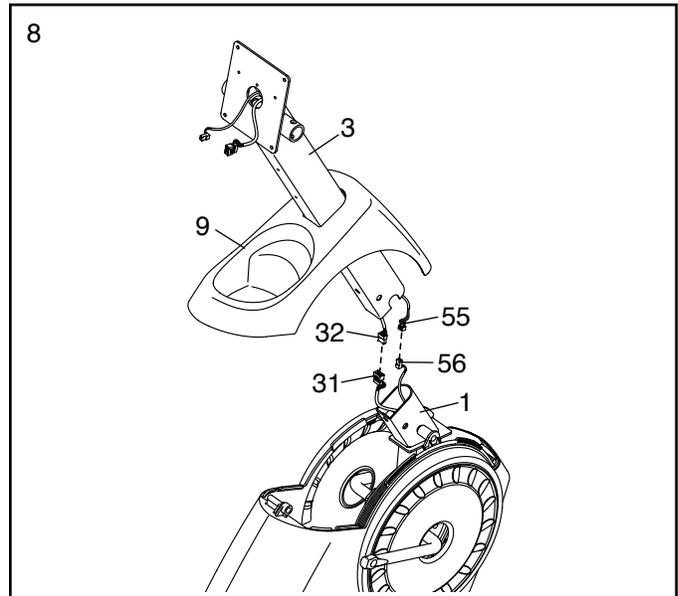
9. **Tip: Avoid pinching the wires.** Slide the Upright (3) onto the Front Frame (1).
