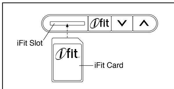
Select the desired workout on the iFit card by pressing the increase and decrease buttons next to the iFit slot. The duration of the workout will appear in the left display, the maximum resistance level for the workout will flash in the center display, and the number of the workout will appear in the right display.
