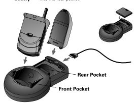
**Note:** If two or three batteries are loaded in the charger, the batteries will charge one at a time. The main battery attached to the phone will charge first, the attached auxiliary second, and the battery in the rear pocket last.
