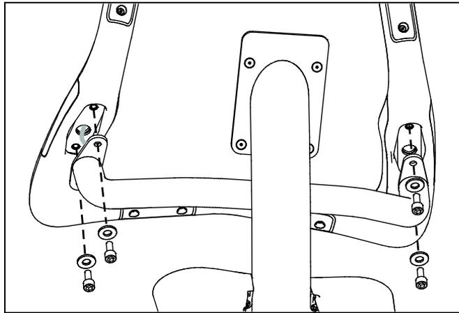
**Figure 8: Installing the handlebars**
