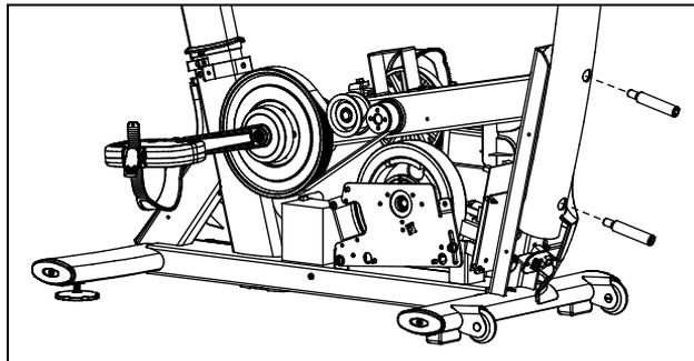
**Figure 6: Bolting the upright support into place**
