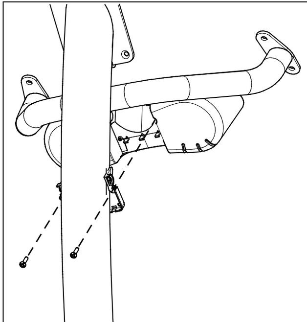
**Figure 7: Installing the bottle holder**
