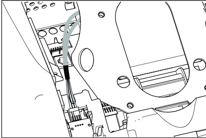
**Figure 14: Connecting the heart rate cable**
