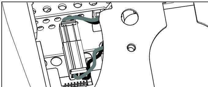
**Figure 15: Connecting the power cable**
