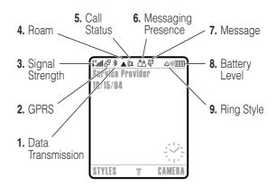
1. Data Transmission Indicator – Show connection and data transmission status. The Bluetooth® wireless connection indicator ≯ shows when a Bluetooth connection is active. Other indicators can include:
