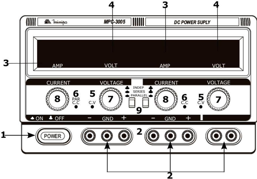
Figura 1 – Painel Frontal Fontes MPC-3003 e MPC-3005
