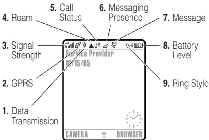
**1. Data Transmission Indicator** – Show connection and data transmission status. The Bluetooth® wireless connection indicator
