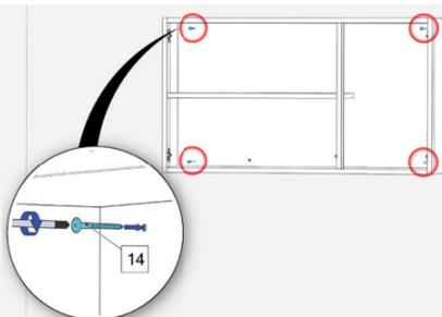
Encaixe as capas dos parafusos (item 13)
