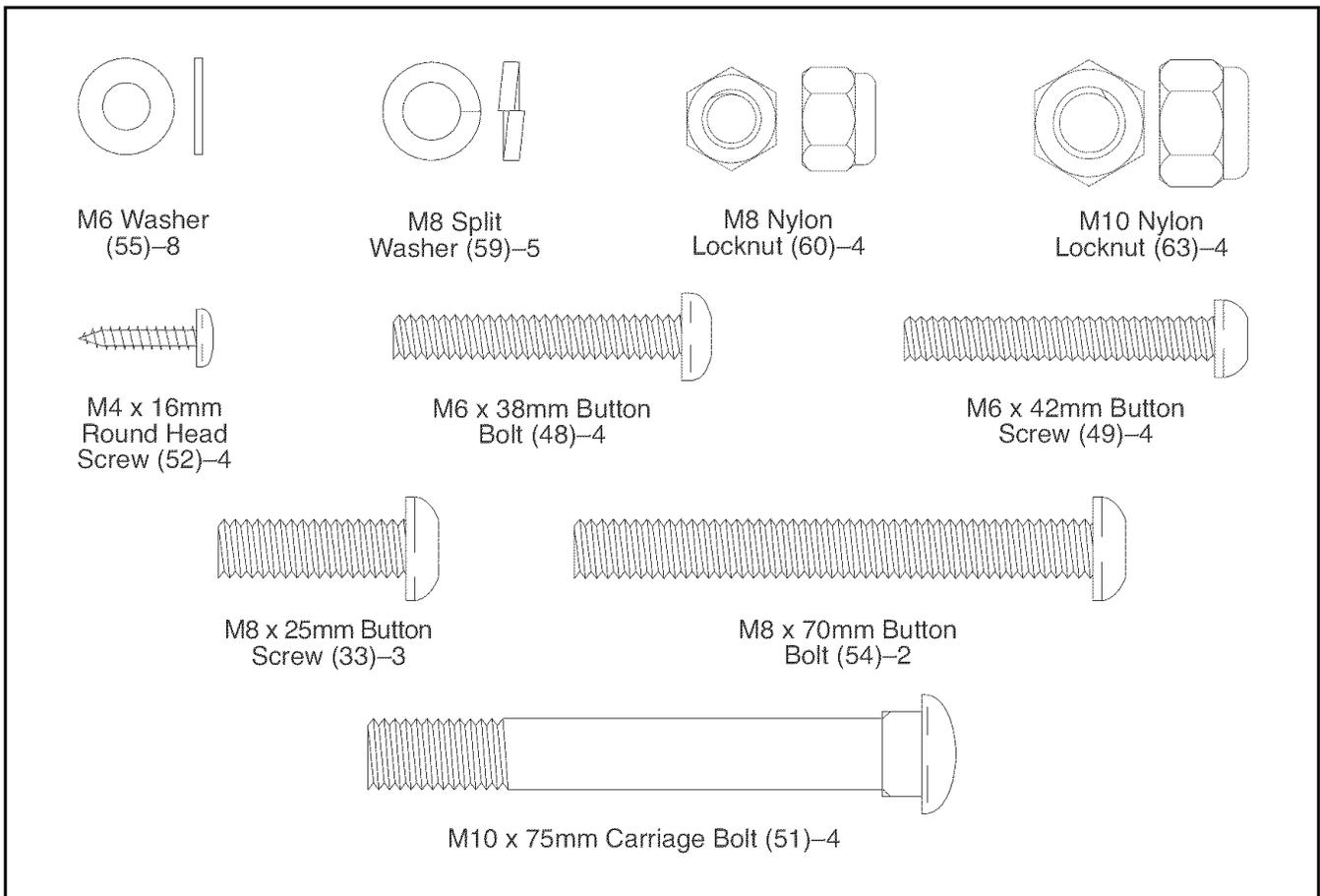
1. While another person lifts the front of the Frame (1) slightly, attach the Front Stabilizer (3) to the Frame with two M10 x 75mm Carriage Bolts (51) and two M10 Nylon Locknuts (63).
