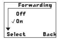
Use the arrow keys to select the desired function and press the soft key directly below **Select**.
