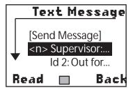
The New Message icon (<n>) appears in front of any new unread messages. To read a message, use the arrow keys to scroll to the desired message and press the softkey below Read on the LCD.
