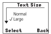
You have two text selections; Normal and Large. Use the arrow keys to highlight your selection and press the softkey directly below **Select** to save the selection and return to the previous menu.
