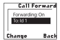
To change or select the Id designated to receive forwarded calls, use the arrow keys to highlight the **To Id** function as illustrated above and press the softkey directly below **Change**.
