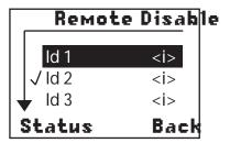
**NOTE:** A  $\checkmark$  next to an Id on the Remote Monitor list indicates that the Id is already selected for remote monitoring.
