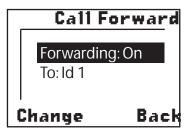
To turn the Call Forwarding function on or off, use the arrow keys to highlight **Forwarding** and press the softkey directly below **Change**. The screen changes to show the **Forwarding** screen.
