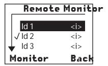
To monitor an Id, use the arrow keys to highlight an Id from the list to monitor. Press the softkey directly below Monitor. The screen changes to show the Id's status as illustrated below.
