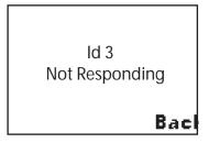
**NOTE:** Remote Monitoring automatically times out after 60 seconds. The screen changes to display the above timeout message for three seconds and returns to the Remote Monitor screen.
