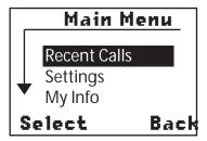
Use the arrow keys to scroll through the available menu options. Highlight the desired menu option and press the softkey directly below **Select**. The screen changes to show the selected view:
