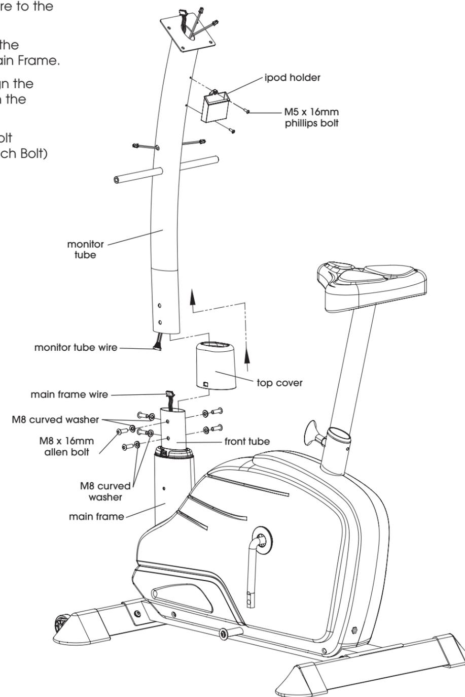
Figure 3 - Installing Monitor Tube
