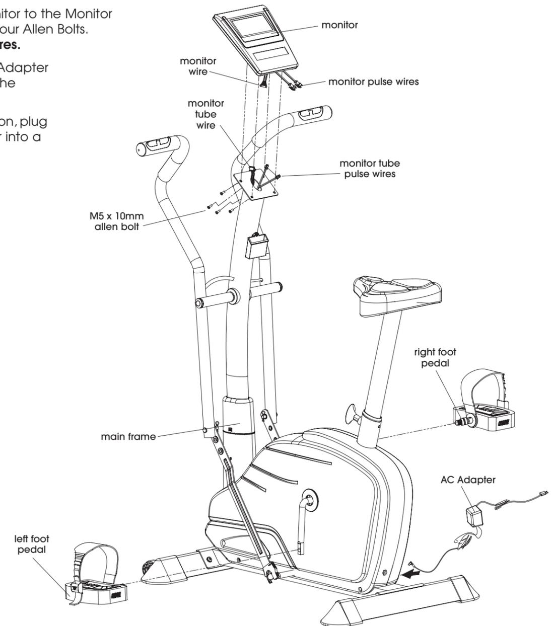
Figure 5 - Install Foot Pedals, Monitor and AC Adapter
