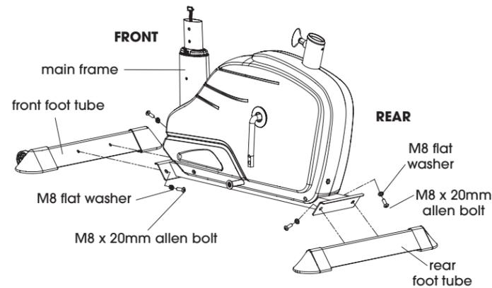
Figure 1 - Install Foot Tubes to Main Frame
