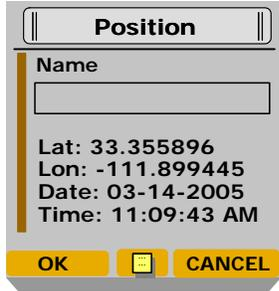
In the *Name* field, type the name you want to use to list the position in your address book, using the GPS unit keypad. If you leave the name blank, the position will be saved with the date and time as the name.
