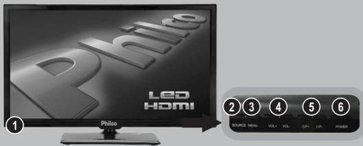
**1** SENSOR DO CONTROLE REMOTO E LED INDICADOR DO STANDBY.
