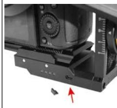
Open the socket to connect the Mini-USB cable
