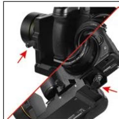
Fasten the screws for secure hold
