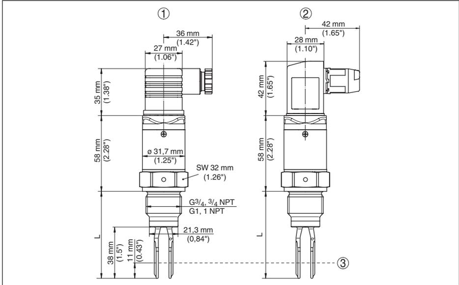
Fig. 33: SITRANS LVL100, modelo padrão - Rosca G $\frac{3}{4}$ , G1 /  $\frac{3}{4}$  NPT, 1 NPT
