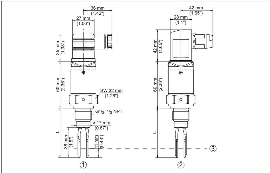
Fig. 32: SITRANS LVL100, modelo padrão - Rosca G $\frac{1}{2}$ ,  $\frac{1}{2}$  NPT
