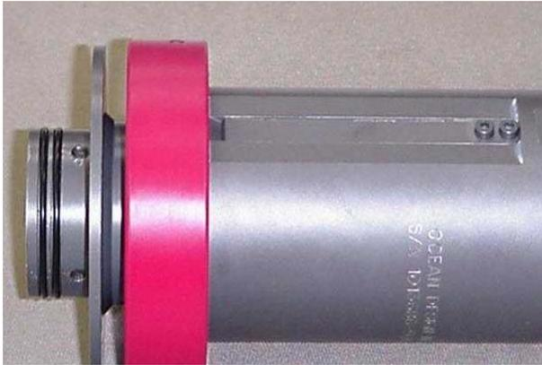
**FOTO 1:** Conector ROV com as garras fechadas
